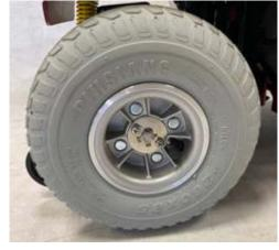
Whenever a centre bolt of the wheel assembly has been loosened, please replace a specified new bolt from an authorised dealer and secure with a torque of  $240 \pm 5$  kg-cm together with Loctite 271 adhesive (or equivalent).
