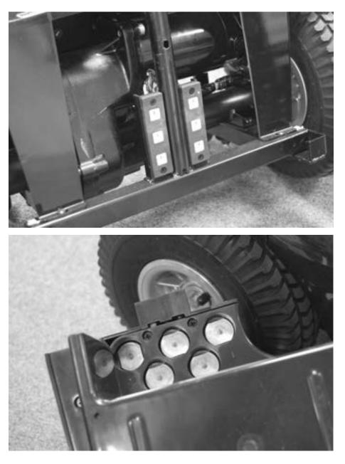
We also recommend that the connectors between the battery pack and the main chassis are also treated at the same time to prevent any carbon build up (round plate connectors and pins). Simply re-assemble the scooter as per user manual after these procedures have been undertaken.
