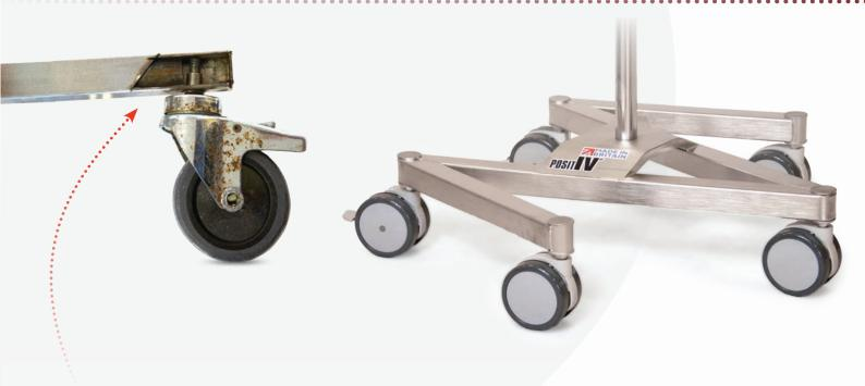
insert and rust tarnished castor fork. The cutaway shows the castor bush has become loose with use.
